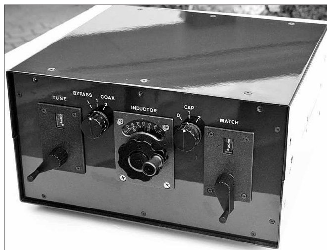
Figure 24.12 — Front panel view of the ARRL Antenna Tuner as built by Lee Jennings, ZL2AL. Lee used vacuum-variable capacitors in the construction of his tuner.
